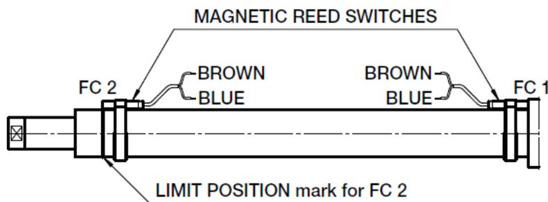
Figure 6.2 – FCM magnetic stroke limit switches
