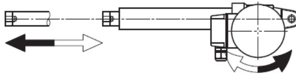
Figure 6.9 – Push rod shifting directions
