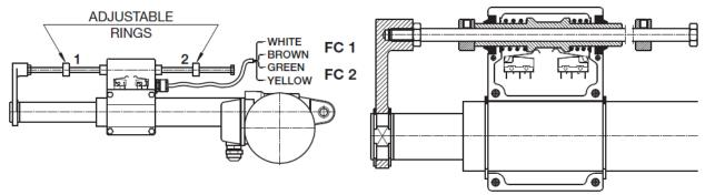
Figure 6.1 – FCE electric stroke limit switches
