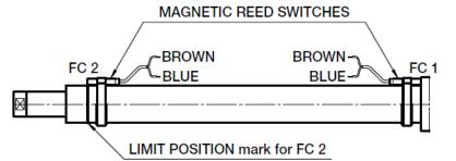
Figure 6.2 – FCM magnetic stroke limit switches
