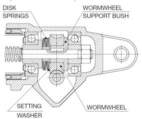
• The torque limiter clutch is preloaded during assembly.
