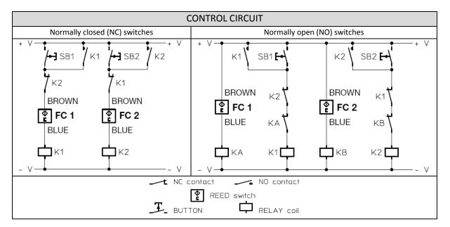
The MAGNETIC LIMIT SWITCHES must be connected to the electric control circuit as shown in the following WIRING DIAGRAM:
