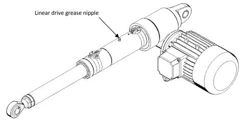
Figure 9.2 – Linear drive relubrication of ACL2/ACL2 B 30-40
