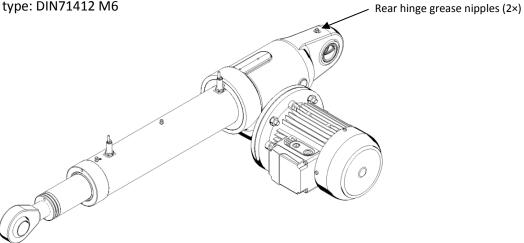
Figure 9.4 – Rear hinge grease nipples
