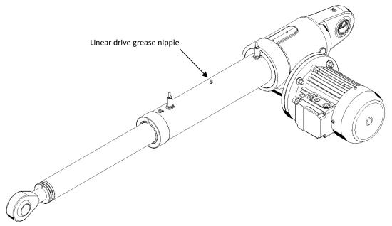
Figure 9.2 – Linear drive relubrication
