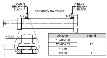
Figure 6.2 – FCP inductive proximity stroke limit switches
